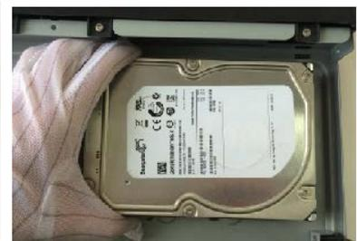
3. Put the HDD into the Device.
