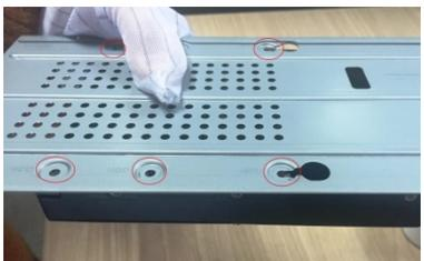
4. Match the holes on the bracket with the screw holes on HDD.
