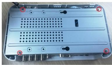
2. Remove the screws to take off the bracket.
