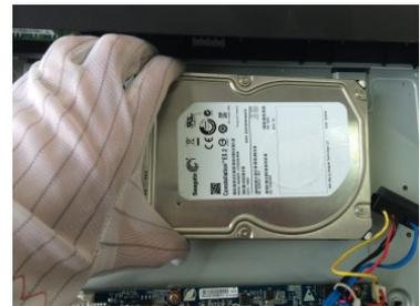
3. Place the HDD onto the Device.
