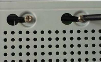
4. Turn the device to see the back side of it. Aim the screws of the HDD at the holes on the back of the device and fix the screws.
