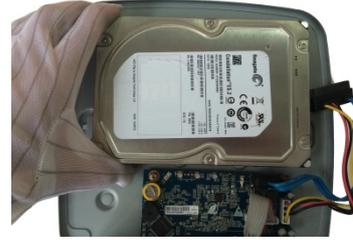
3. Match the screws with the holes on the DVR (WITHOUT HDD) (WITHOUT HDD) to place the HDD.
