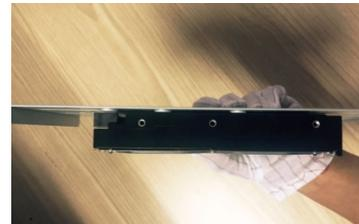
3. Put the HDD onto the bracket.
