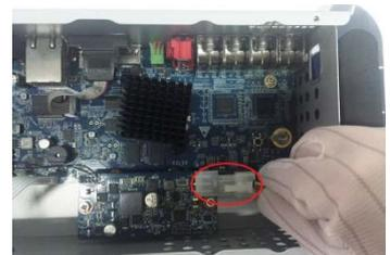
6. (Optional) Put the battery cable through the hole to connect into the cable port.
