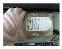
3. Place the HDD onto the Device.
