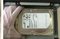
3. Put the HDD into the Device.
