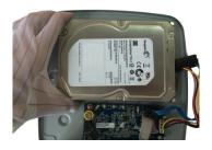
Match the screws with the holes on the DVR (WITHOUT HDD) (WITHOUT HDD) to place the HDD.
