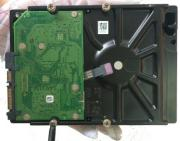
2. Fix the screws on the HDD but do not be fastened.
