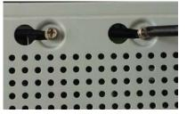
Turn the device to see the back side of it. Aim the screws of the HDD at the holes on the back of the device and fix the screws.
